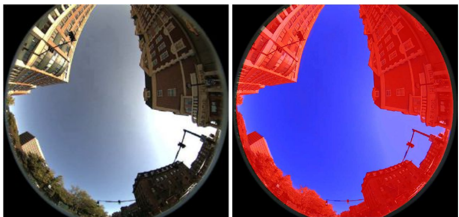
(a) An exemplary hemispheric image (b) An overlay consisting of the original and the binary categorization into sky and obstruction
